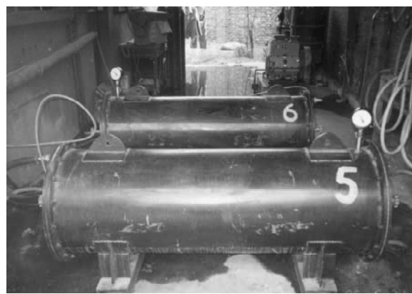
Fig. 1. The hydride container of 80 \text{m}^3 (under standard conditions) hydrogen capacity.
