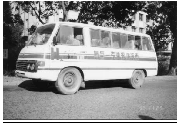
Fig. 6. The 19 seater gasoline hydrogen hybrid powered minibus.
